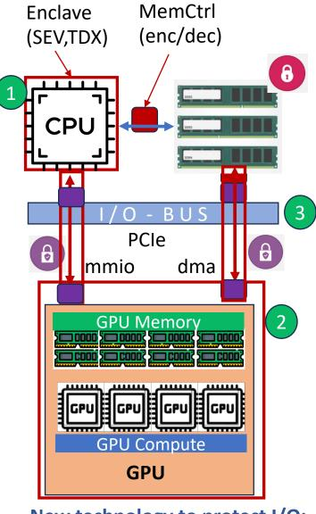
New technology to protect I/O: SPDM: link encryption TDIO: dma access with mem key TDISP (PCIe-5) <sup>15</sup>
